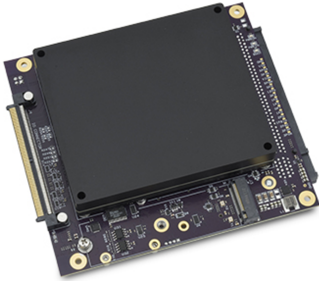
Osbourne with AGX Orin module installed
