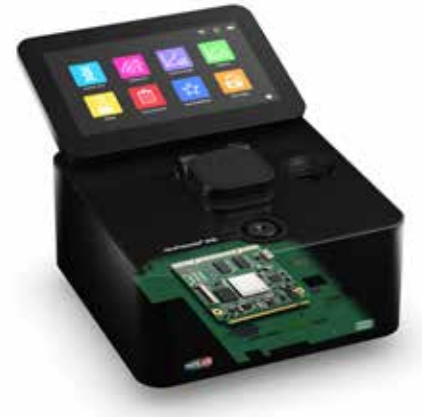
Computer-on-Module based designs get the customization via the carrier boards. This offers the same benefits as full custom designs but incurs far less engineering costs.
