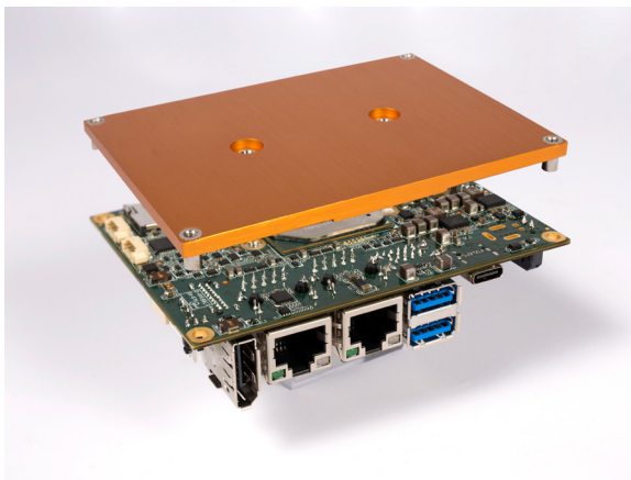
The CPU sits on the underside of the Congatec Pico-ITX SBC. Fanless passive cooling solutions dissipate the waste heat directly to the housing, resulting in a robust system with a long service life and MTBF without moving parts.
