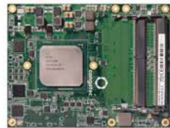
The new Server-on-Modul from in the COM Express Type 7 specification integrates Intel Xeon processors (Codename Broadwell DE)
