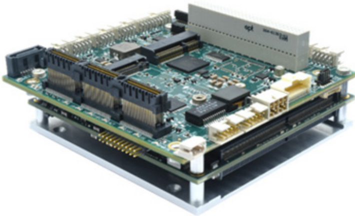
GEMINI complete solution with COM, memory, and heat spreader installed
