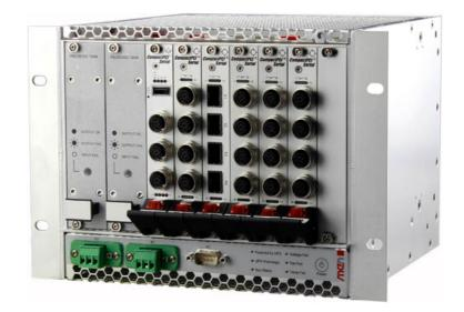
The NH30 is a modular turn-key network switch solution with carrier grade Layer 2 and Layer 3 VLAN routing capabilities offering a seamless throughput of 29 Gbit/s. It is designed for use in trains, trams or industrial environments.
