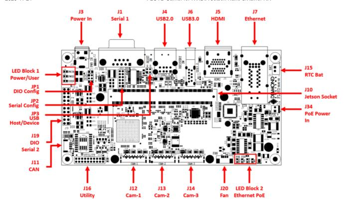
Note: Mini PCIe and M.2 2280 sockets are located on the bottom side.
