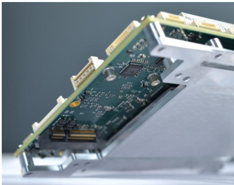
Second MiniCard socket available on bottom
