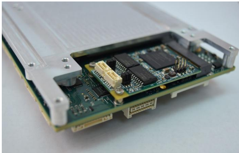
Bottom of Venus SBC showing easy access to optional inserted PCI minicard in the cutaway portion of the heat spreader.
