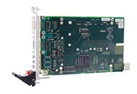
The board is designed and tested for the railway and industrial market, but may be used for other industrial applications, too. It provides 3 USB 3.0 ports and isolated RS232 and RS422/485 interfaces, for either service or continuous operation in a railway or industrial environment.
