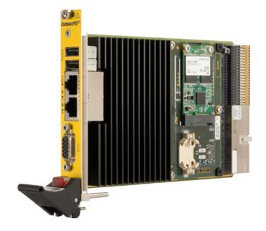
The CPs are designed to run a deterministic real-time operating system such as the QNX<sup>®</sup> Neutrino RTOS Safe Kernel or PikeOS. It is also possible to implement diversitary software on both kernels. All three CPUs support Linux and QNX<sup>®</sup>.
